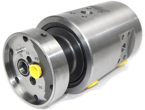
BGB have designed and manufactured two variants of joint, the "Sealed" type where the chambers are separated with specially designed seals, and the "Hydrostatic" type, that does not require seals between chambers.
