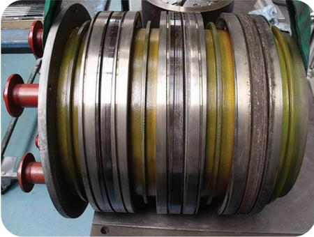
BGB can repair, refurbish or replace all types of slip rings. The refurbished slip ring will be returned to a similar “as new” condition, even if the slip ring is physically damaged.
